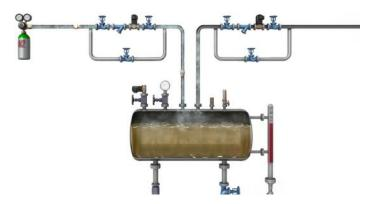
**Oxygen Exclusion:** Oxygen is a key factor in the degradation and oxidation of the thermic fluid. By blanketing the expansion tank with nitrogen, the oxygen is displaced, minimizing the contact between the fluid and the air. This helps to prevent the oxidation and thermal degradation of the thermic fluid.
